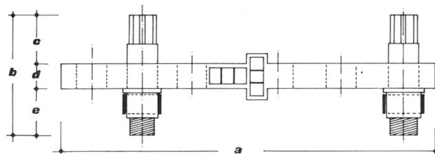
a= mm. 300 | b= mm. 95 | c= mm. 40 | d= mm. 20 | e= mm. 35 | h= mm. 50
